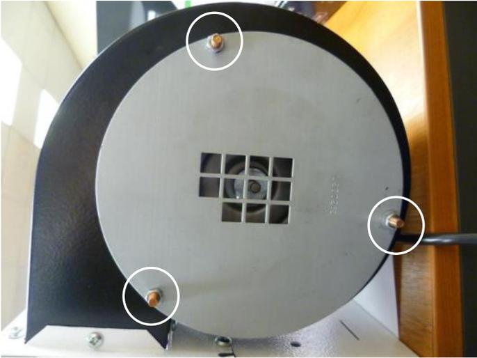
Step 2: Do **not** remove the orifice plate. Attach the fresh air inlet plate over the fan studs and refasten with the original nuts, making sure not to cross thread the fan stud fixings.
