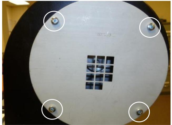
Step 2: Do **not** remove the orifice plate. Attach the fresh air inlet plate on top of the orifice plate and refasten with the original screws, making sure not to cross thread the fan fixings.
