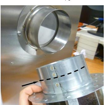
Step 5: Push the wind and rain hood cover fully home, then using a 3mm bit, drill 2 pilot holes either side of the spigot in the horizontal plane.
