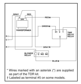
Figure 2. Wiring Diagram for Air Handler Applications.
