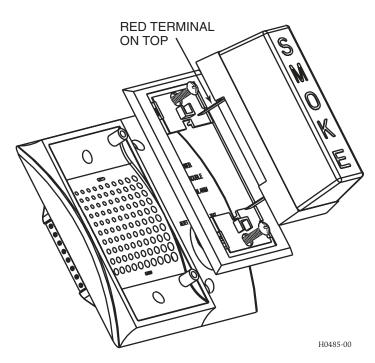
The PS24LO strobe will be mounted on top of the sounder, on the left-hand side of the SSK451. Place one mounting spacer between the SSK451 and the strobe adapter plate at each screw attachment location. Attach the adapter plate, spacer and SSK451 to the left-hand side of the double-gang electrical outlet box with two mounting screws.
