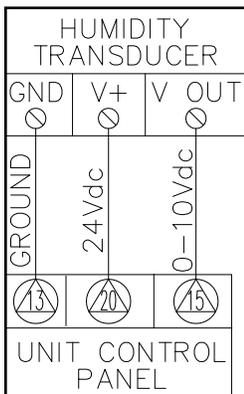
**NOTE:** Terminals 13, 15, and 20 are typical control panel terminals and should be verified on the unit specific wiring diagram.
