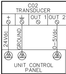
**NOTE:** The same ground reference has to be used for the CO2 Sensor and for the DDC/signal receiver. Terminals 20, 26, and 28 are typical control panel terminals and should be verified on the unit wiring diagram.
