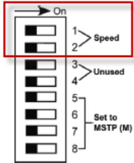
**Baud rate legend is printed on the IQ cover. For default 9600, both SW1 and SW2 are set to OFF.**
