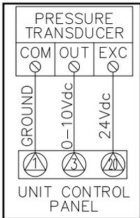
**NOTE:** Terminals 1, 3, and 20 are typical control panel terminals and should be verified on the unit specific wiring diagram.
