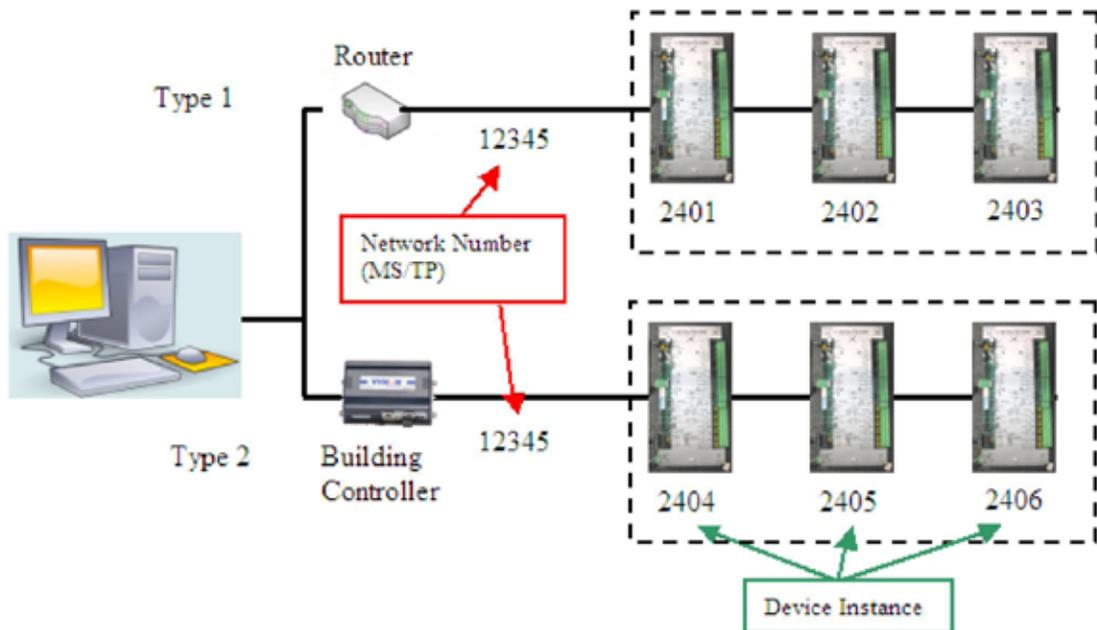
**Illustration Type 1** - The first type uses a **router** to connect the controllers to the main building automation system computer. These are networks typical of Automated Logic, Siemens, Delta controls, and Reliable controls. A network of this type requires that all MSTP field bus wiring have a unique Network number. It also requires that all controllers connected have a unique device instance. This is for all systems and buildings connected to the Building Automation System.
