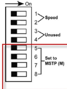
**The protocol legend is printed on the IQ cover. For MS/TP, set SW5, SW6, SW7, and SW8 to OFF for either master(m) or slave (s).**
