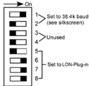
Set the switches according to the legend on the IQ cover. (Set SW5 to ON; set SW6, SW7, and SW8 to OFF.)
