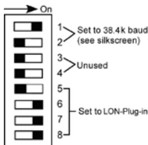
Baud rate legend is printed on the IQ cover. For LonWorks, set switches for 38.4k bps. (Set SW1 to ON; set SW2 to OFF.)
