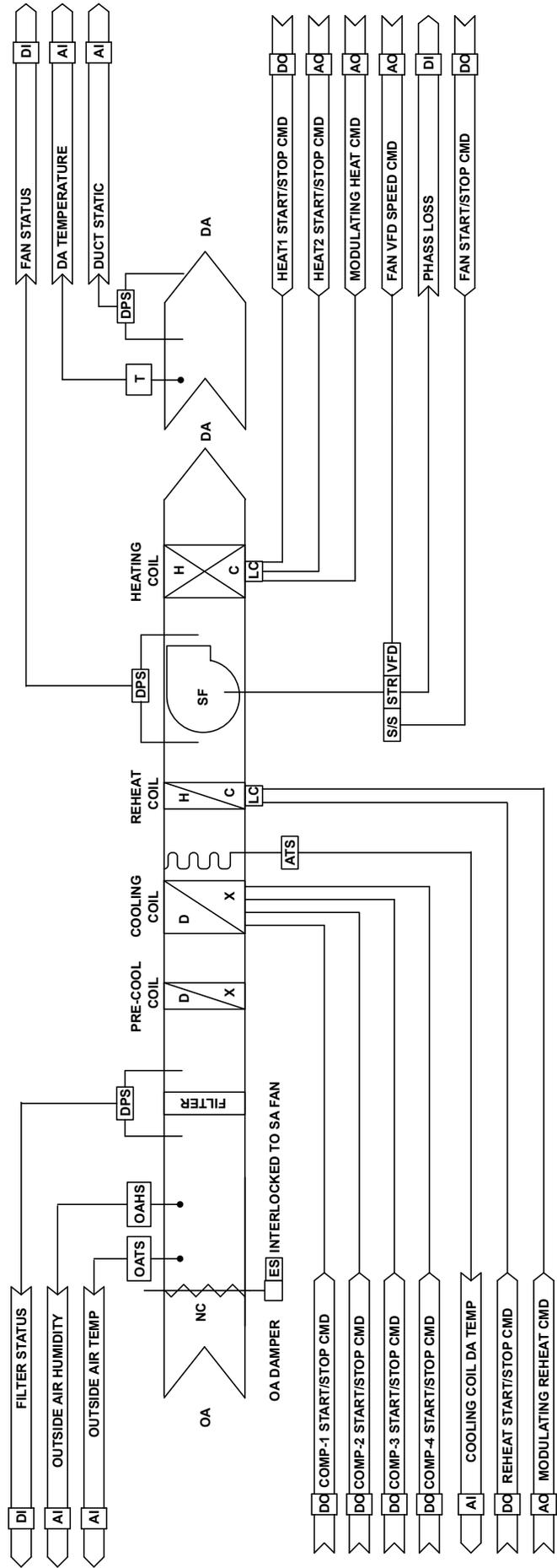
**TYPICAL AIR FLOW SCHEMATIC**
