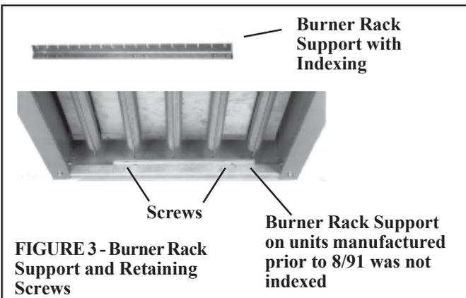
**To Remove the Burner Rack** -- With the burner rack assembly "hanging" down, lift up on the rear and slide the assembly up and out of the manifold support brackets.
