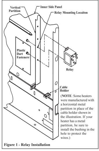
Hold the relay in line with the holes and attach it with the two plastic fasteners.
