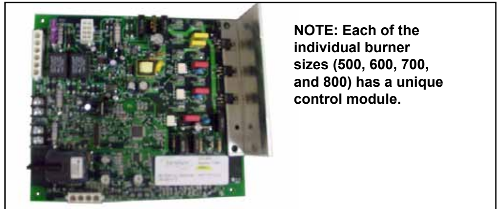
FIGURE 43A - Control Module used in Modulating Gas Control Option AG70 - "D" Cabinet only
