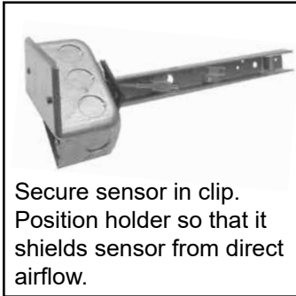
FIGURE 38 - Discharge Air Sensor Holder, PN 115850, used in Makeup Air Installations
