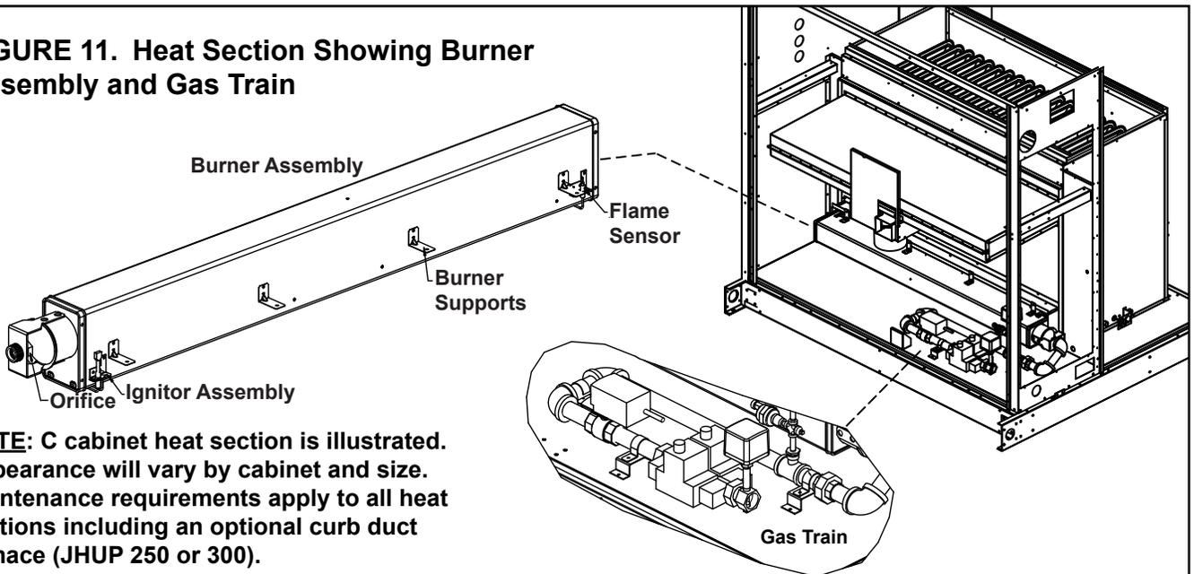
**NOTE:** C cabinet heat section is illustrated. Appearance will vary by cabinet and size. Maintenance requirements apply to all heat sections including an optional curb duct furnace (JHUP 250 or 300).
