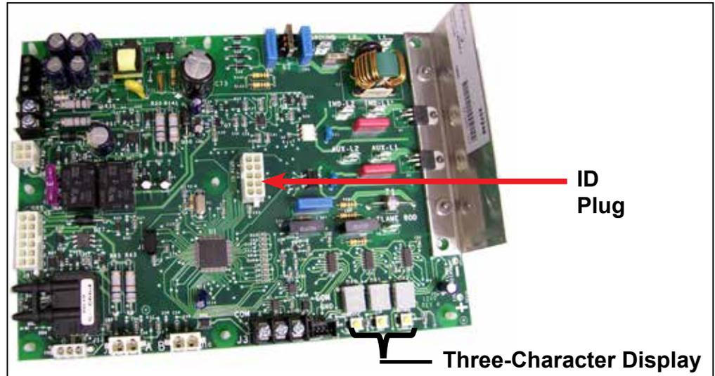
The control has a built-in, self-diagnostic capability. The control continuously monitors its own operation and the operation of the heat section including direct spark ignition, safety and modulating valves, and venter motor speed. The three-character display on the control indicates the current system state, warnings, failures, and test modes.
