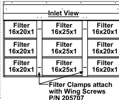
**Instructions:** Remove filters by loosening the wing screws and sliding the filter clamp(s). Clean with soap and water, allow to dry, and replace. If it is more convenient to keep an extra clean set of filters, quantities, filter sizes, and part numbers are listed.
