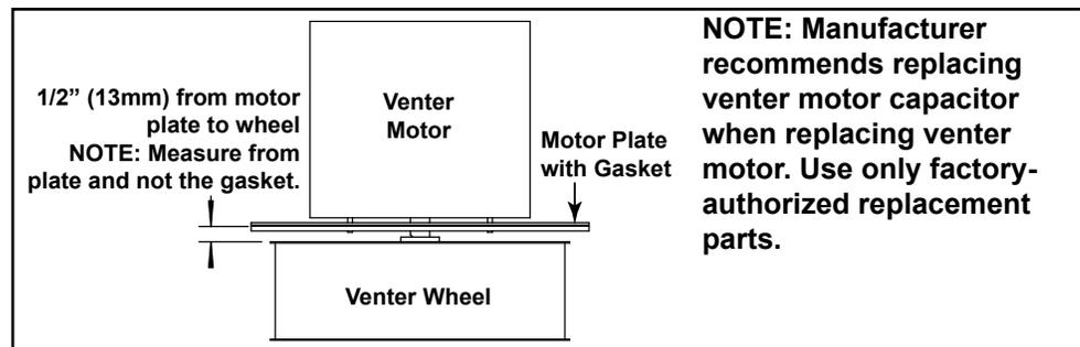
If replacing venter parts, see **FIGURE 3** for proper spacing. If the motor plate gasket is damaged or deteriorated, replace it with **PN 222856**.
