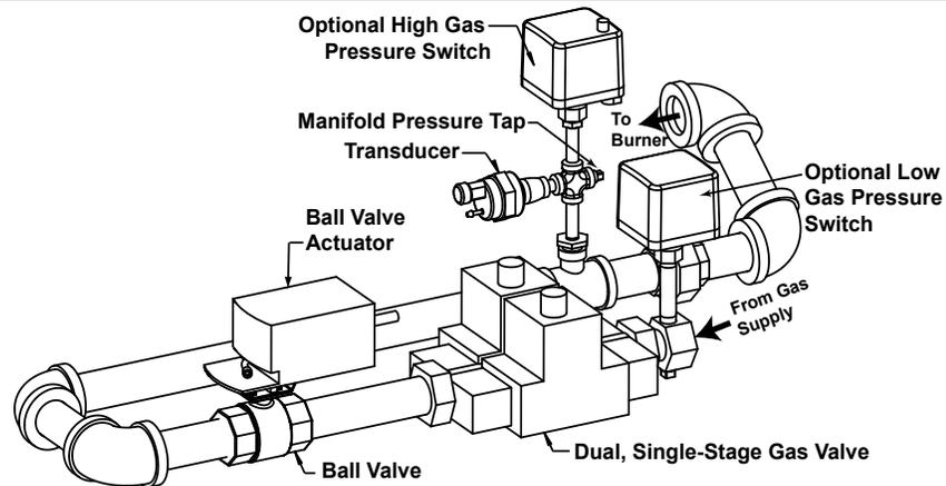
**Single-Stage Operating Gas Valve:** All gas trains have either a single-stage or a dual single-stage safety gas valve. The gas valve must be checked annually to ensure that it is shutting off gas flow completely; follow the instructions in box below.
