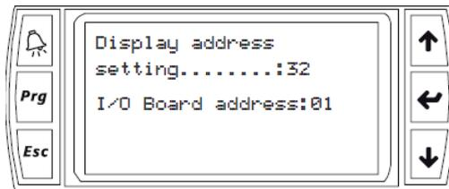
To change the address of the terminal ("Display address setting"), proceed as follows. Press the ENTER button once: the cursor will move to the "Display address setting" field. Select the desired value using the UP and DOWN buttons, and confirm by pressing ENTER again. If the value selected is different from the value previously saved, the following screen will be displayed and the new value will be saved to the permanent memory.
