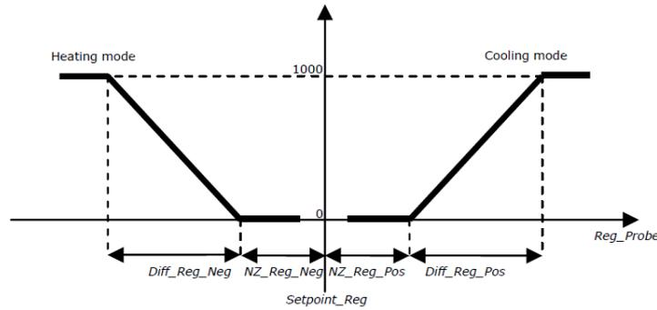
With this type of control, when return temperature reaches the set point, all the heating and cooling elements are off. All the heating or cooling elements will be on when reaching set point + differential.
