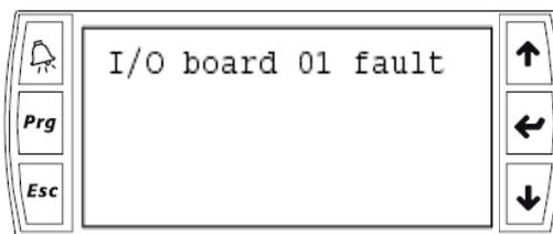
If the terminal detects the inactivity of the entire pLAN network, that is, it does not receive any message from the network for 10 consecutive seconds; it cancels the display completely and shows the following message:
