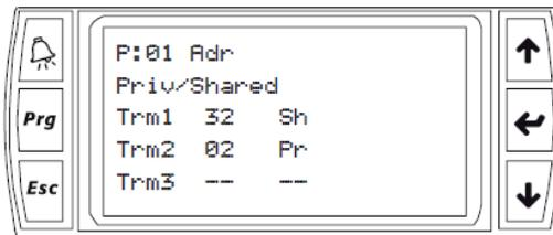
Change the configuration of the terminals as required. The ENTER button is used to move the cursor from one field to another, while the UP and DOWN buttons change the value of the current field. P:xx shows the address of the selected pCO board (in the example shown in the figure, this is board 1).
