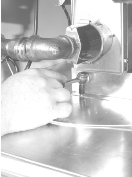
Figure 20 Remove 2 screws of the burner slider
