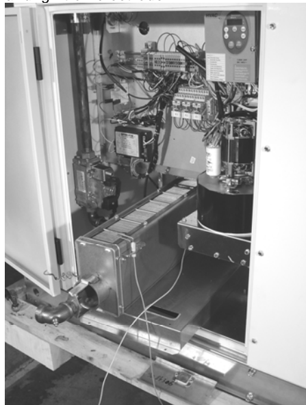
Figure 24 Remove burner box (together with flame sensor and ignition electrode)
