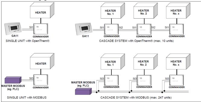
Possibilities: • Set the state of the heater(s) (OFF – VENTILATION – HEATING)
