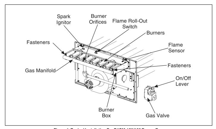
Figure 1. Typical Installation For R4GM-150/180 Burner Box
