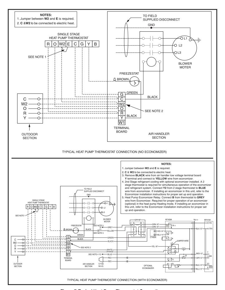
Figure 7. Typical Heat Pump Thermostat Connections
