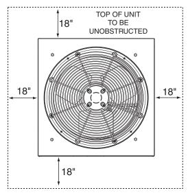
Figure 2. Clearance Requirements
