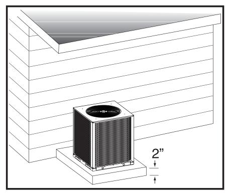
Figure 3. Ground Level Installation
