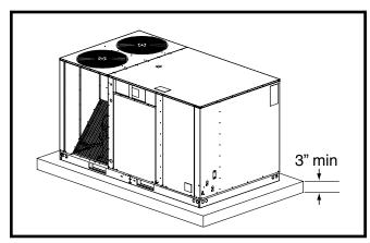
Figure 7. Concrete Pad Installations
