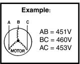
2. Determine the average voltage in the power supply.
