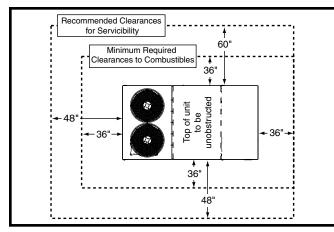
Figure 1. Minimum Clearances to Combustibles
