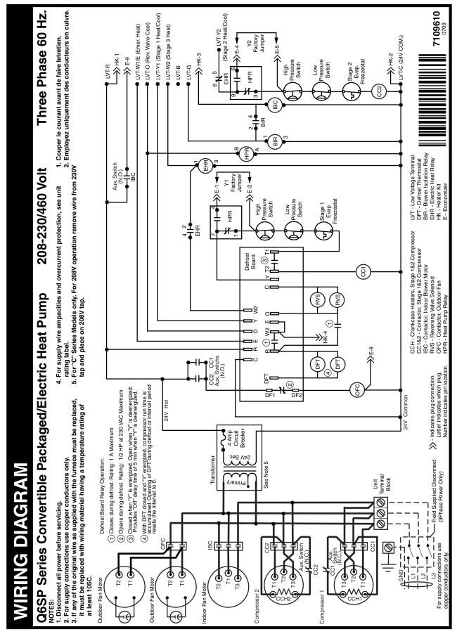
Figure 11. Ladder Diagram for Q6SP-090/120 (C/D) Series
