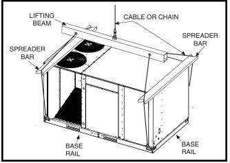
Figure 5. Rigging & Hoisting
