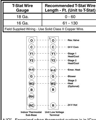
‡ "O" - Energized when thermostat system is in "Cool" Mode.
