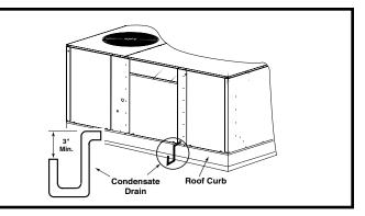
Figure 2. Condensate Drain
