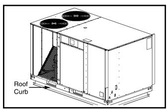
Figure 6. Roof Curb Installations
