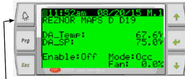
**Option RB5 or RB6 Remote Display Flashing Alarm Key**
