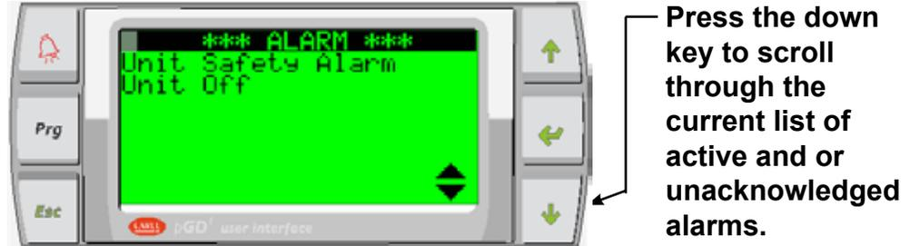
When you reach the end of the queued alarm list, you will be prompted to either press the alarm key to clear the alarms or press the enter key to display the alarm logger.
