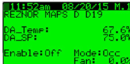
2. Press the Program Key to access the main menu and then press the up or down arrow keys to navigate to the **A. Quick Setpoints** submenu. Press the enter key to select.
