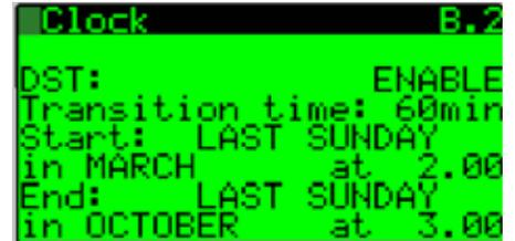
From **Screen B.2**, press the enter key to access the modifiable DST fields and set the values accordingly.
