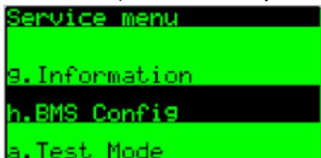
3. From the BMS Config screen E.h.1 verify that the Protocol: field is set to Bacnet MSTP. On a BAS card retrofit the Protocol: field may need to be set. To change the protocol press the enter key until the cursor is flashing on the Protocol: field and use the up or down key to scroll through the available choices and select Bacnet MSTP then press enter to confirm the protocol change.
