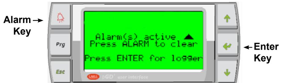
Pressing the enter key will display the first page of the alarm logger. The first page of the alarm logger will contain the most recently logged alarm with a date, time, Alarm ID and a snapshot of the OA Temp, OA Humidity, DA Temp, CC Temp, and MA Temp sensors at the time the alarm was logged. Pressing the up key in succession will display any remaining logged alarms from the most recent to least recent entry.
