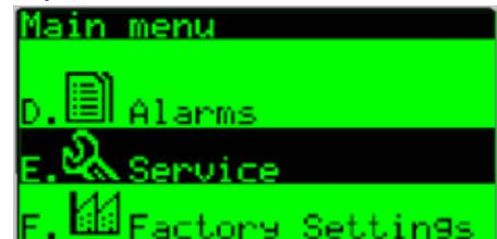
When prompted to enter the Service Password, use the up or down arrow keys and enter the service password of 7125, and press the enter key.
