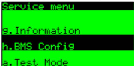
3. From the BMS Config screen E.h.1 verify that the Protocol: field is set to Lon. On a BAS card retrofit the Protocol: field may need to be set. To change the protocol press the enter key until the cursor is flashing on the Protocol: field and use the up or down key to scroll through the available choices and select Lon then press enter to confirm the protocol change.
