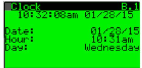
3. Once set, press the enter key in succession until the cursor is blinking in the uppermost left hand corner of the screen and press the down arrow key to advance to **Screen B.2**.
