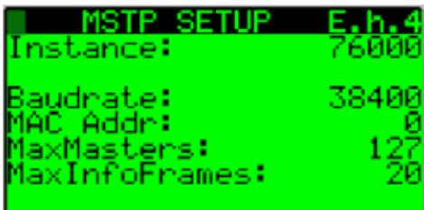
Press the enter key in succession until the cursor is flashing in the uppermost left hand corner of the screen and use the down arrow key to navigate to the next screen.
