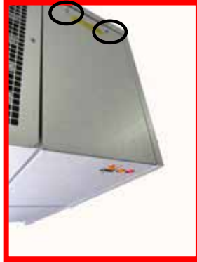
FIGURE 8. Remove two lid retaining screws (indicated in circles shown) located on the right hand side on the top of the air curtain cabinet.
