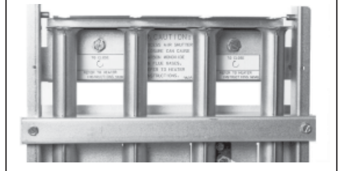
Figure 18 - Air Shutter Adjustment Screws -- Alternate Turning Screws When Adjusting Shutter
