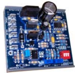
FIGURE 34 - Signal Conditioner, P/N 134170, used in Option AG57, Gas Controls with 6:1 Turndown
