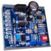
FIGURE 20B - Signal Conditioner in Option AG21
