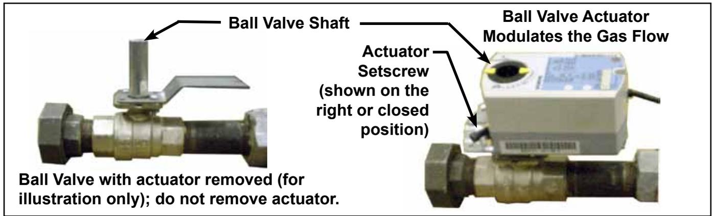
**Modulating System Gas Valve (Ball Valve & Actuator) Adjustment**
