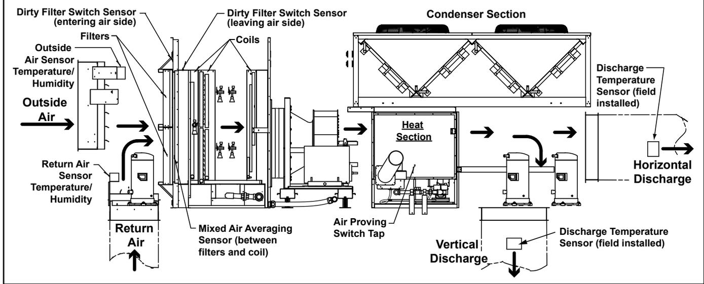
**Service:** If a sensor needs to be replaced, use only a factory authorized replacement part designed for the purpose. Refer to the digital wiring requirements in Paragraph 7.4 of Installation Form I-MAPSIII&IV).
