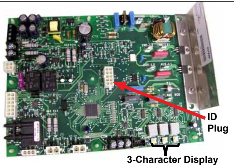
The control has a built-in, self-diagnostic capability. The control continuously monitors its own operation and the operation of the heat section including direct spark ignition, safety and modulating valves, and venter motor speed. The 3-digit display on the control indicates the current system state, warnings, failures, and test modes.
