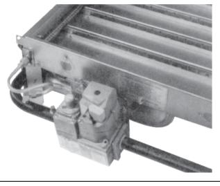
**10.** Insert the carryover orifice into the lighter tube. If fit is tight, lightly tap the orifice into position.
