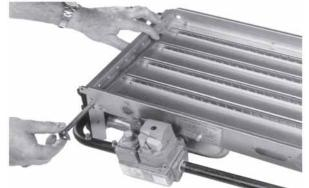
5. Install drip shield. NOTE: "Z" effect when observed from the side. Compress lighter tube into half circle cutouts in the burner tubes. Be sure the tube is seated. The 90° angle on the drip shield should be against the top and side of the burner rear plate.
