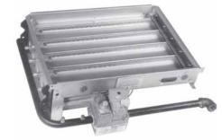
2. Back off screws that attach the manifold to the burner rack. Remove top screws.
