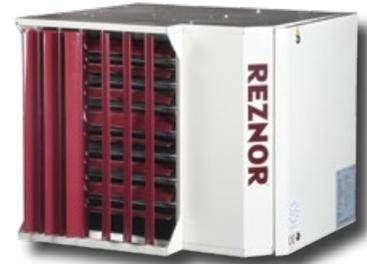
The UDSA (axial fan, free blowing) and UDSBD (centrifugal fan, ducted) achieve 92% thermal efficiency and incorporate a unique 4-pass heat exchanger manufactured from titanium stabilised aluminised steel for enhanced life expectancy.
